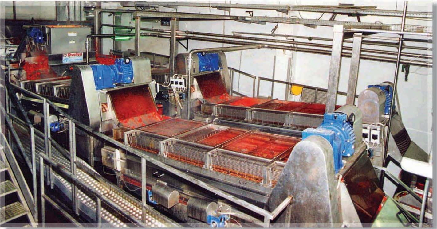
Pre-peel removers and peel removers in series
