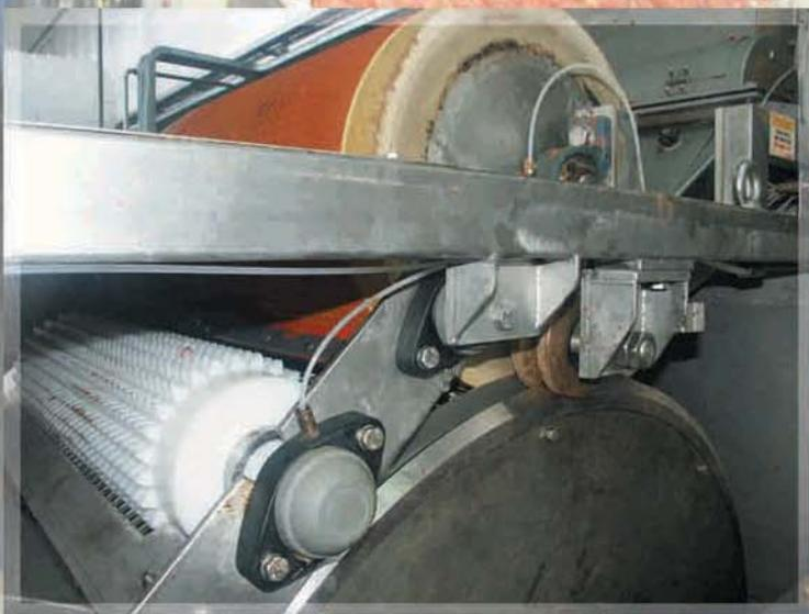
Ejecting roller and pressure roller on the drum
